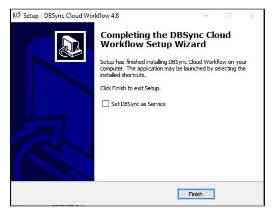
Note: You can also use DBSync as a service by placing a checkmark in the checkbox - as shown above.
